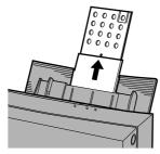
2. Select the paper feed mode by switching the paper feed switch to position "A".
